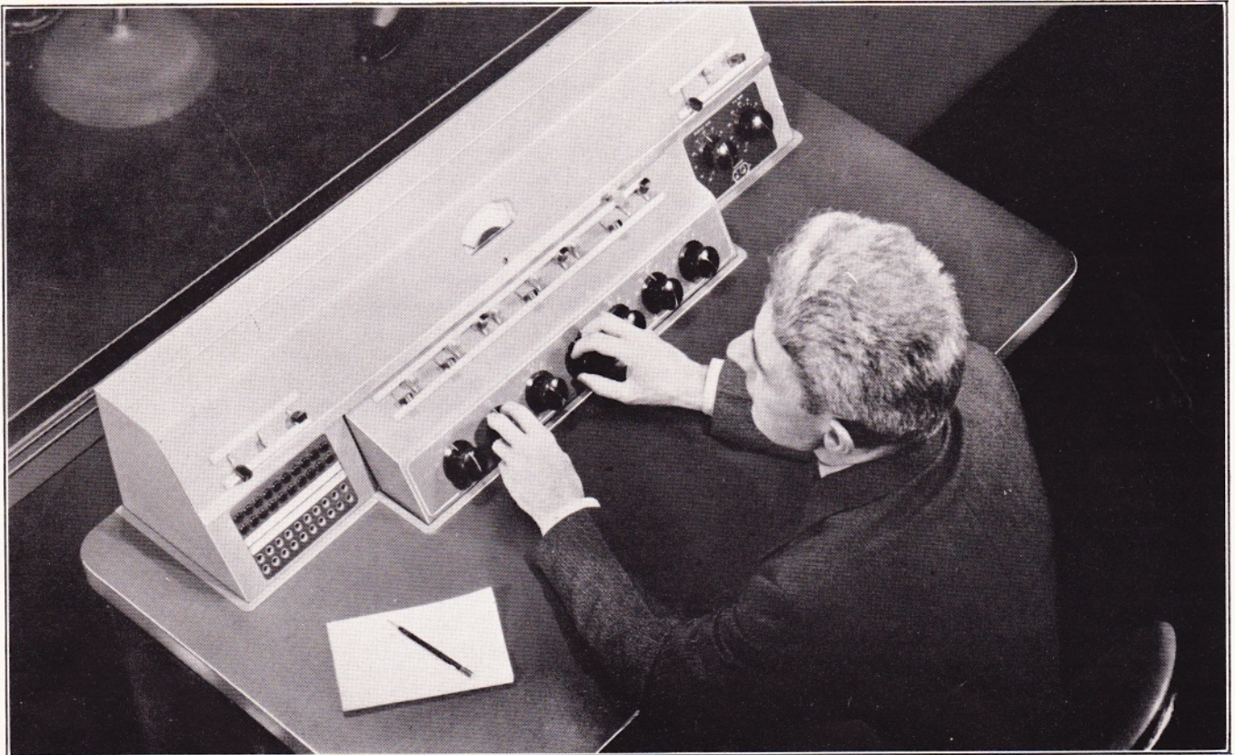
FIG. 2, ABOVE. The seven control knobs across the lower front are, from left to right, line mixer, four microphone mixers, and master gain controls for each of two channels. Talk-back key and line mixer transfer key are above the line mixer.
